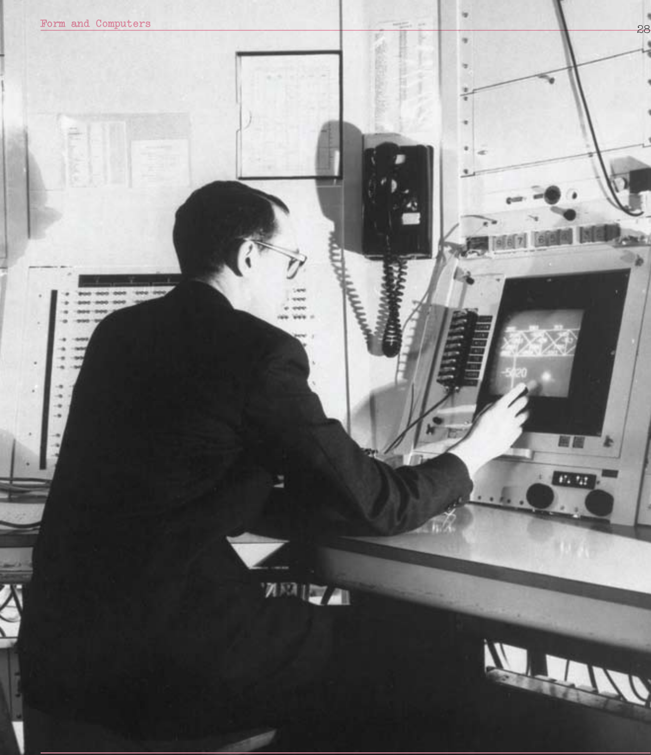
Sketchpad , Ivan Sutherland, 1963. With Sketchpad, users drew directly on the screen using a light pen. The behavior of
