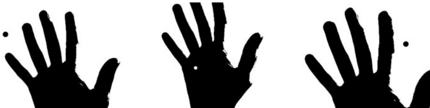
Example 3. Distinguishes the silhouette of people or objects in each video frame by comparing each pixel to a threshold value. The circle is filled with white when it is within the silhouette.
