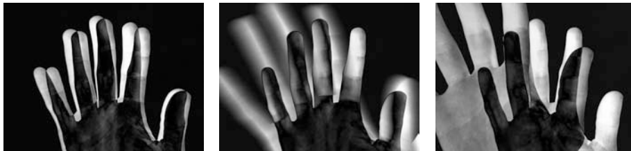
Example 2. Detects the presence of someone or something in front of the camera by comparing each video frame with a previously saved frame. The change is visualized and is calculated as a number.
